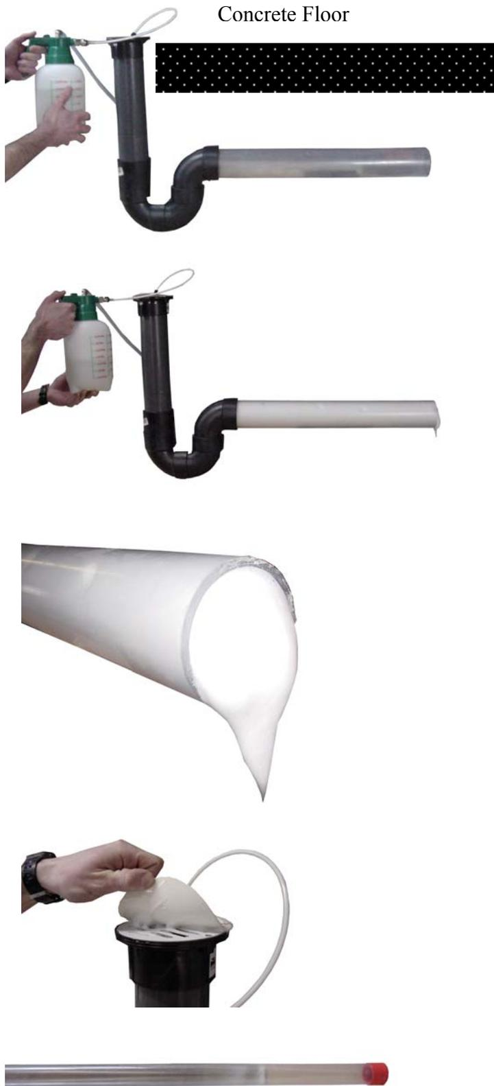
Floor drain tests have been completed to record time and volume. The picture shows a standard drain complete with trap. This is a 4-inch diameter pipe with an overall length of 62 inches. From the top of the drain pipe inlet to bottom of the trap is 19 inches.
